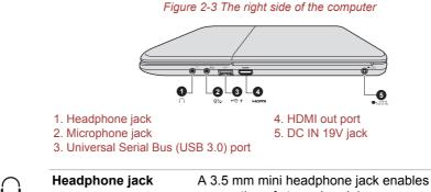
⊕<sup>z</sup><sub>z</sub> Microphone jack A 3.5 mm mini microphone jack enables connection of a three-conductor mini jack for stereo microphone input.
